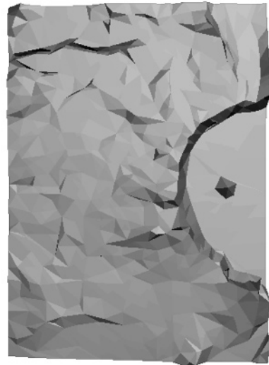
Figure 13: Simplified model with 999 faces (took 46 seconds).
