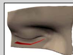
transfer of the deformations from the coarse tetrahedral mesh onto the triangular mesh
