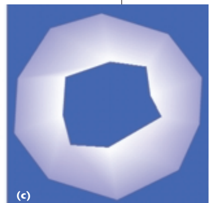
4 Preserving genus limits drastic simplification. The original model of a brake rotor with (a) 4,736 triangles and 21 holes is simplified with a topology-preserving algorithm using (b) 1,006 triangles and 21 holes and a topology-modifying algorithm with (c) 46 triangles and one hole. Model courtesy of the Alpha_1 Project, University of Utah.
