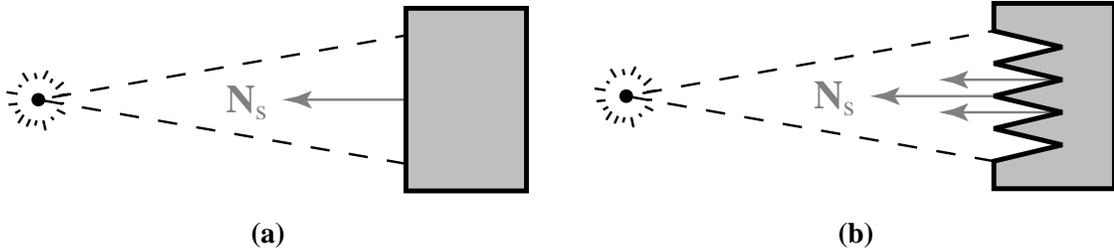
**Figure 5.9:** (a) A flat, diffuse surface facing toward a point light source, with  $\mathbf{N}_s = \mathbf{N}_g$ . The surface is assumed to not to absorb any light, so that the incident and reflected power is the same. (b) A ridged surface with shading normals that point toward the light. It receives the same power as (a), but reflects far more due to its larger surface area.
