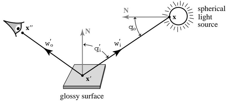
**Figure 9.1:** Geometry for the glossy highlights computation. The radiance for each viewing ray is obtained by integrating the light that is emitted by the source, and reflected from the glossy surface toward the eye.
