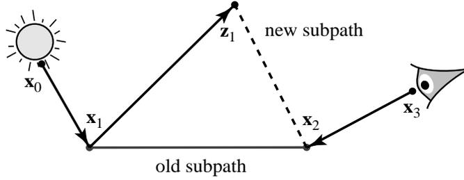
**Figure 11.3:** A simple example of a bidirectional mutation. The original path  $\bar{x} = x_0 x_1 x_2 x_3$  is modified by deleting the edge  $x_1 x_2$  and replacing it with a new vertex  $z_1$ . The new vertex is generated by sampling a direction at  $x_1$  (according to the BSDF) and casting a ray. This yields a mutated path  $\bar{y} = x_0 x_1 z_1 x_2 x_3$ .
