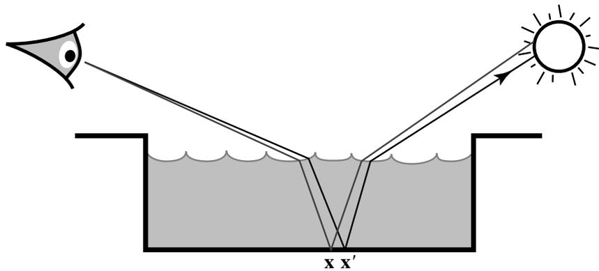
**Figure 11.6:** Using a two-chain perturbation to sample caustics in a pool of water. First, the lens edge is perturbed to generate a point  $x'$  on the pool bottom. Then, the direction from original point  $x$  toward the light source is perturbed, and a ray is cast from  $x'$  in this direction.
