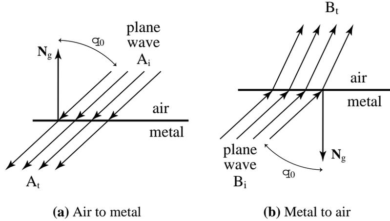
**Figure 6.2:** When absorbing media such as metals are present, the path of a light beam is not always reversible. For example, when a light beam  $A_i$  is transmitted from air into some metals, there is a non-zero angle of incidence  $\theta_0$  for which the beam does not change its direction of propagation (Figure (a)). However, a beam of light  $B_i$  traveling in the reverse direction (from metal into air) is refracted at the surface, and follows a different path (Figure (b)).
