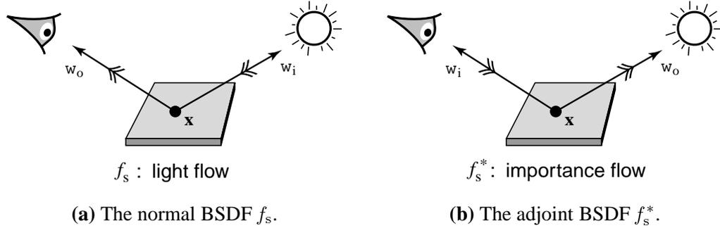
**Figure 3.3:** By adopting the convention that  $\omega_i$  is always the sampled direction, the BSDF  $f_s$  and its adjoint  $f_s^*$  are used for different purposes. **(a)** The BSDF  $f_s(\omega_i \rightarrow \omega_o)$  is used for radiance evaluation, and to scatter importance particles. **(b)** The adjoint BSDF  $f_s^*(\omega_i \rightarrow \omega_o)$  is used for importance evaluation, and to scatter light particles.
