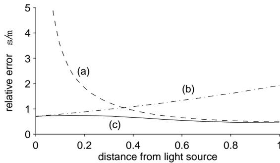
**Figure 9.13:** A plot of the relative error  $\sigma/\mu$ , as a function of the distance from the light source. Three curves are shown, corresponding to the three images of Figure 9.12. The curves have been normalized to show the variance when  $n_1 = 1$  and  $n_2 = 2$  (the same ratio of samples used in Figure 9.12).
