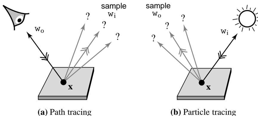
**Figure 3.2:** Path tracing and particle tracing sample the BSDF in different ways. **(a)** For path tracing, the direction  $\omega_o$  is given (it points toward the previous vertex on a path leading to a sensor). The path is extended by sampling a direction  $\omega_i$  according to the BSDF. **(b)** For particle tracing, the direction  $\omega_i$  is given (pointing along a path toward a light source), and the path is extended by sampling a direction  $\omega_o$ .
