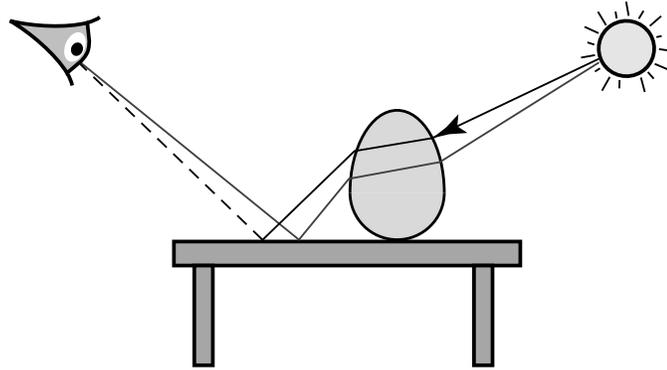
**Figure 11.5:** A caustic perturbation. A new path is generated by perturbing the direction of the ray from the light source by a small amount, and then tracing the perturbed ray through the same sequence of specular reflections and refractions as the original path.
