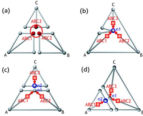
**Figure 5:** Virtual Nodes for a progressive face subdivision
