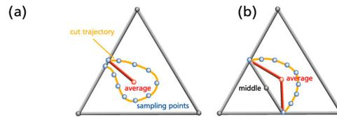
**Figure 10:** Sampling for midface node position: (a) turning point, (b) face midpoint
