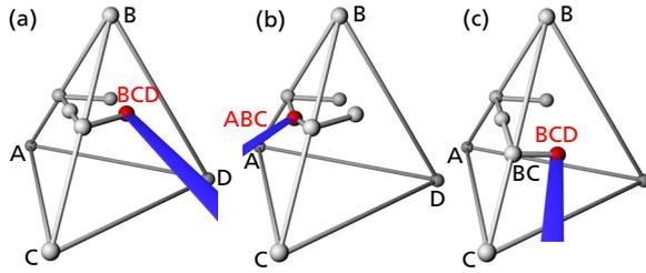
**Figure 9:** Trembling over edges: (a) first edge cut, (b) backwards movement, second edge cut, (c) forward again, third edge cut
