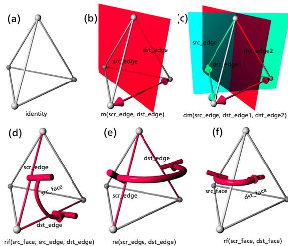
**Figure 6:** Transformations: (a) identity, (b) mirror, (c) double mirror, (d) rotate inside face, (e) rotate over edges, and (f) rotate over faces
