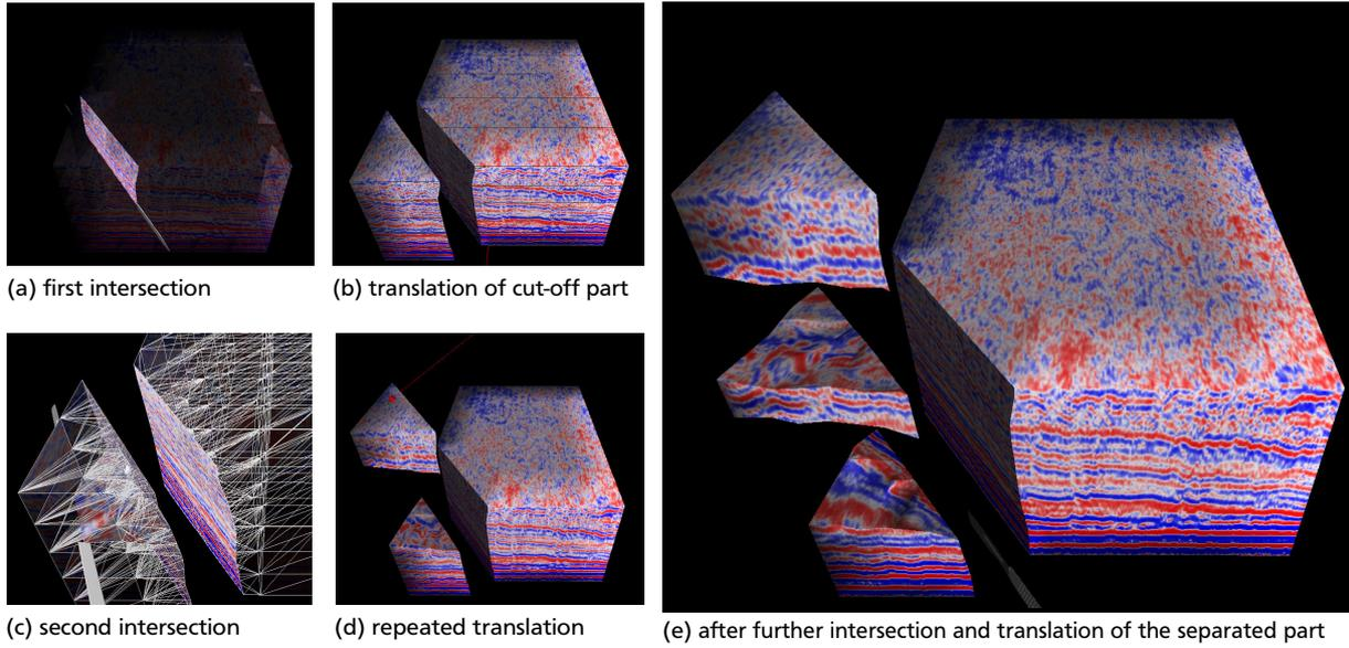
**Figure 14:** *Interactive visualization of a seismic volume data-set*
