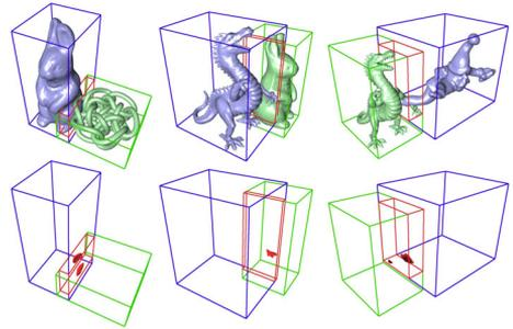
Figure 7: Computation of the intersection volume. AABBs, Vol, and intersection volume are shown for three examples with simple intersections.
