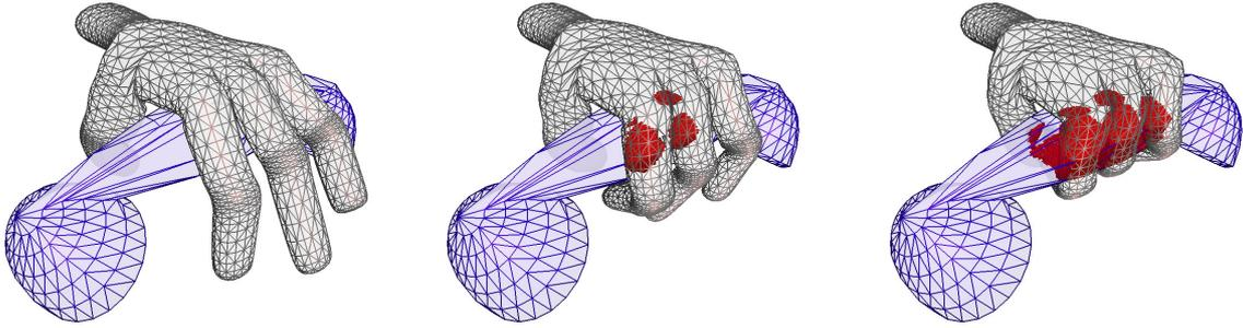
Figure 3: Dynamic animation of a hand with 4800 faces and a phone with 900 faces. Collisions (red) are detected. Refer to Tab. 1 for performance measurements.
