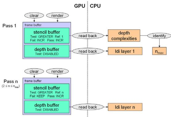
Figure 2: Each rendering pass generates an unsorted LDI layer. Additionally, the first rendering pass computes the depth complexity, i. e. the number of rendering passes.
