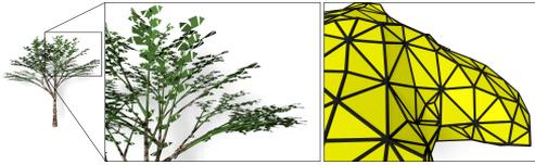
Figure 11: Generating a tetrahedral mesh for an unconnected triangle soup. In this case, the resulting volumetric representation corresponds to the space that is intuitively occupied by the model. The mesh consists of 3K elements.
