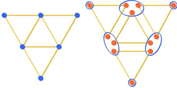
**Figure 1:** A set of mass points with a defined topology represented with basic primitives i.e. triangles (left). All mass points are replaced by constraint sets that contain a number of mass portions (right). The number of mass portions in a constraint set depends on the number of adjacent primitives.
