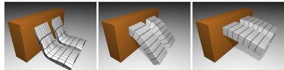
**Figure 4:** Two cuboids with identical geometry are simulated using constraint sets (left) and mass points (right). In the three images, the Young's Modulus is varied from  $5\text{kN/m}^2$  (left),  $500\text{kN/m}^2$  (middle), to  $5000\text{kN/m}^2$  (right). The Poisson ratio is always 0.3.
