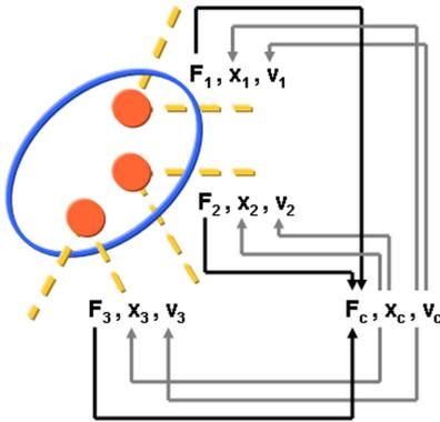
**Figure 2:** Forces  $F_i$  computed at the mass portions are accumulated in a constraint set. After a topology change, position  $\mathbf{x}_c$  and velocity  $\mathbf{v}_c$  are communicated to all mass portions in the constraint set.
