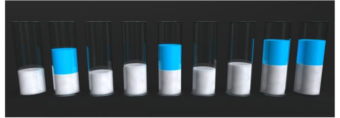
Fig. 3. Compression test with three different settings and three cylinders per setting. The three cylinders on the left show snow with  $E = 20$  kPa, the three cylinders in the middle contain snow with  $E = 140$  kPa and the three cylinders on the right use an IISPH implementation instead of our compressible pressure solver.
